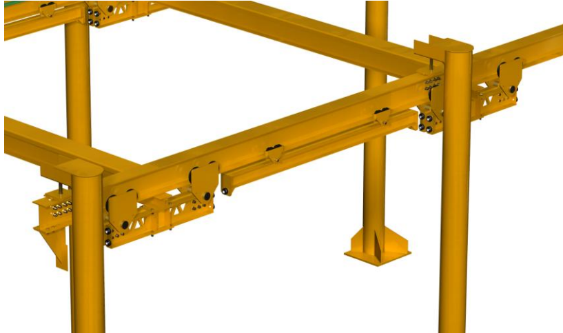
fig. 3.5.2 makes sure both bridges and rolling buffers are push clear to the end of the system against the bridge stops. This will prevent the threat of the bridges rolling toward the open end before the remaining bridge stops can be installed.
