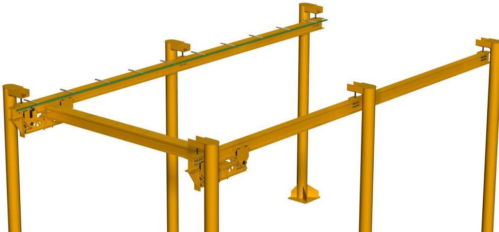
fig. 3.5.1 make sure all endtruck wheels are making proper contact with the runway before removing any rigging from the bridge.
