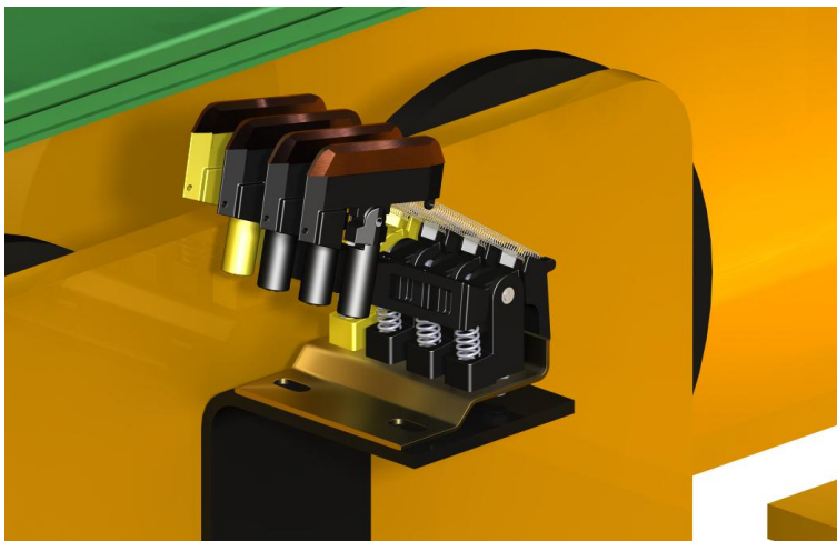
fig. 3.6.5 Make sure the yellow shoe on the collector is in line with the yellow on the buss bar track. Failure to do so may result in buss bar damage and/or power loss.
