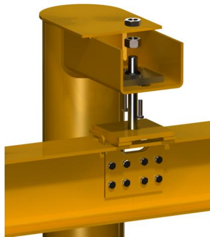
fig. 3.3.2 make sure all hardware has been hand tighten before removing the rigging from each runway.
